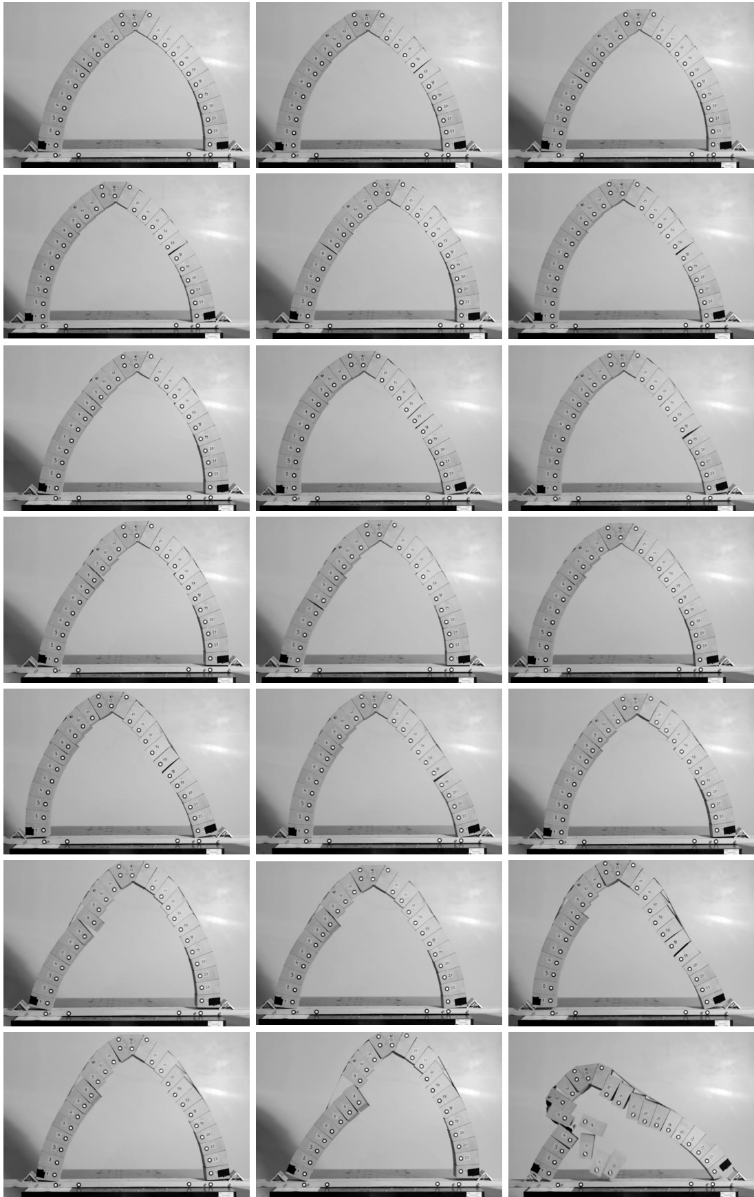
Figure 10: Series of photos documenting testing of pointed arch strengthened at extrados.
